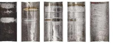
Our EASD In-Pipe system is a cost-effective decontamination method of a flexible design able to treat isolated plant areas commonly found on a nuclear plant. the system can be implemented during the nuclear site decommissioning phase. the technology gives the opportunity for controlled electrical and chemical conditions to enable metals to be decontaminated for free release. Meaning minimised waste volumes, which, in turn, provides significant cost savings.
