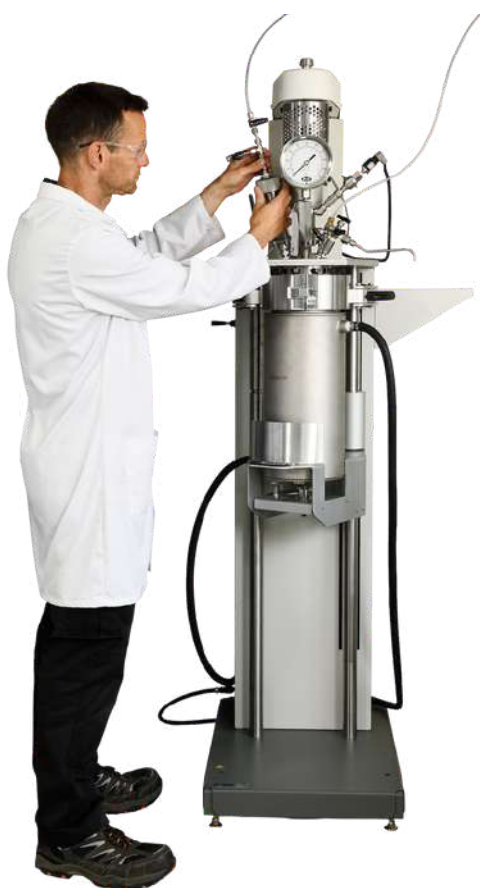
Photo shows the 5 kg reaction vessel designed and used in the work.
