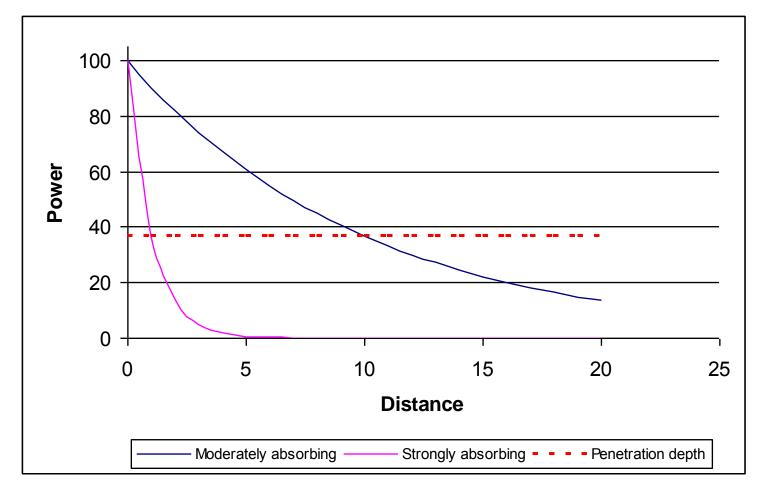
Penetration Depth = Distance through the object being heated where the incident power drops to 1/e of that at the surface
