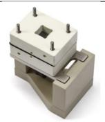
Place brass Current Collector onto Electrode. Fit Insulating Disc and Insulating Sleeve onto the Current Collector.
